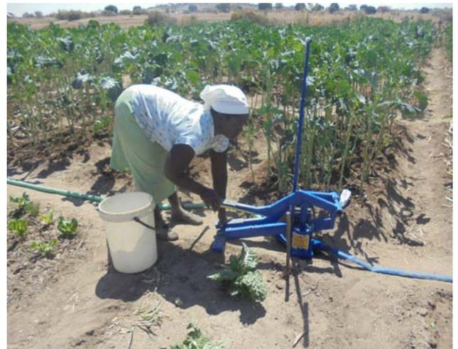
Low cost irrigation pump in use in Gutu
